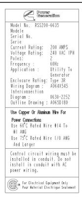
FIGURE 6. RSS200 WITH CONTROL DISPLAY NAMEPLATE
