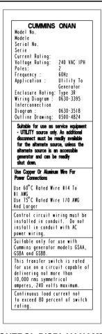
FIGURE 8. RSS200 WITHOUT CONTROL DISPLAY NAMEPLATE, ONE CIRCUIT BREAKER
