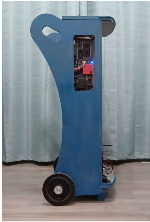
Access for inverter connections
